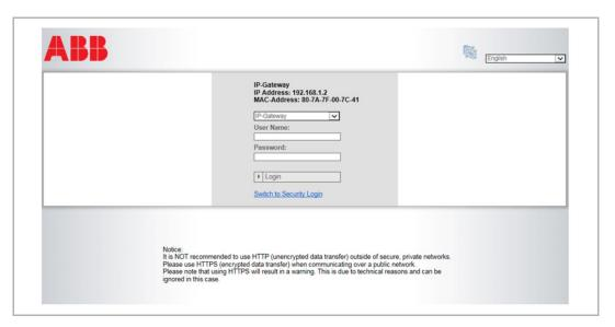
The IP address shows you the IP address currently used by the device.
