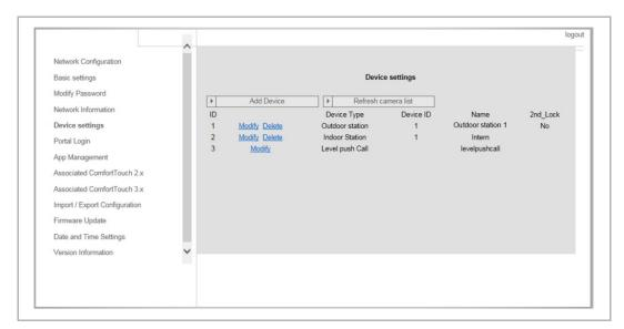
All outdoor stations to be connected to the IP gateway (max. 9) must be listed in the Device settings.
