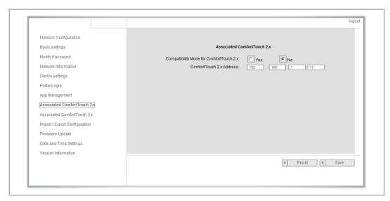
The IP gateway can be used to control Busch-ComfortTouch® of the series 2.x. The Busch-ComfortTouch® firmware must be version 2.4 or higher.
